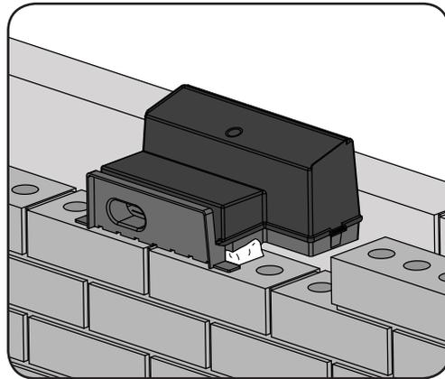
3. Bed the product into position, ensuring that the front edge is flush to the brickwork and the central drainage hole aligns with the perp joint of the course below.
