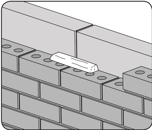
2. Lay a small bed of mortar along the back edge of the course directly below where the swift brick will sit.
