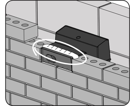
6. Continue bricklaying as normal, up to and over the product. Utilise the channel in the top of the product as a mortar key for the course above.
