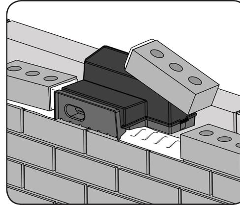
5. Lay the mortar bed for the adjacent bricks, butter the ends and bed them against the product on top of the side support tabs.
